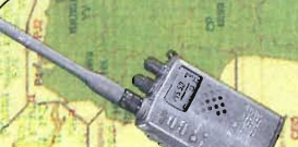
IC-11 - Tribanda palmare 5W VHF 140-470 MHz UHF 400-450 MHz.
